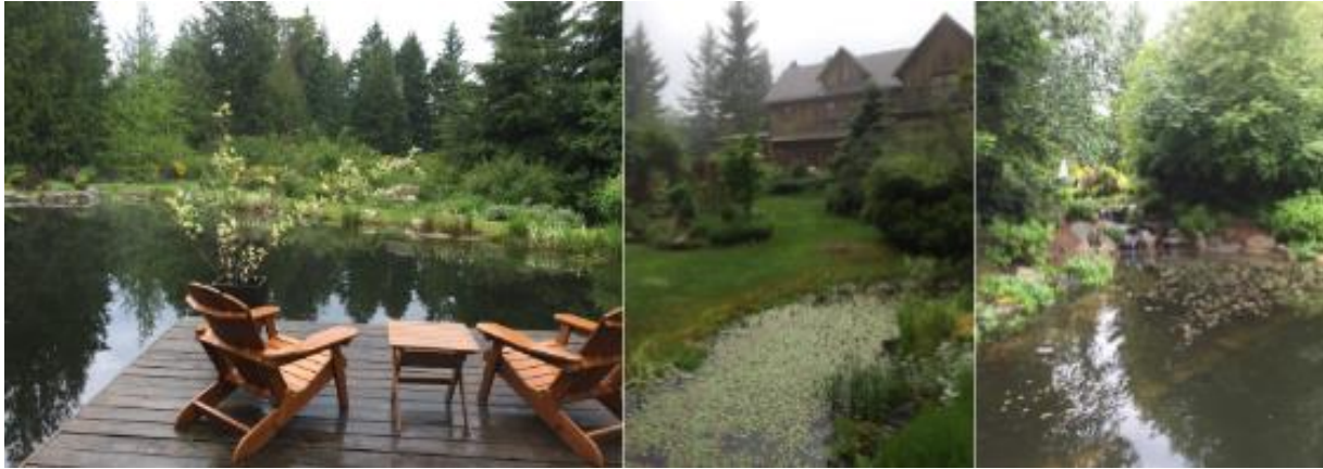
Figure D2. Case study B2 images taken by Kendra Anderson during site visit on May 30, 2017 to gather further details on RWH systems that exist on SSI. Rainwater is collected in the $170,000 pond which has a capacity of 300,000 gallons. This harvested rainwater is used for irrigation of gardens and the property.
